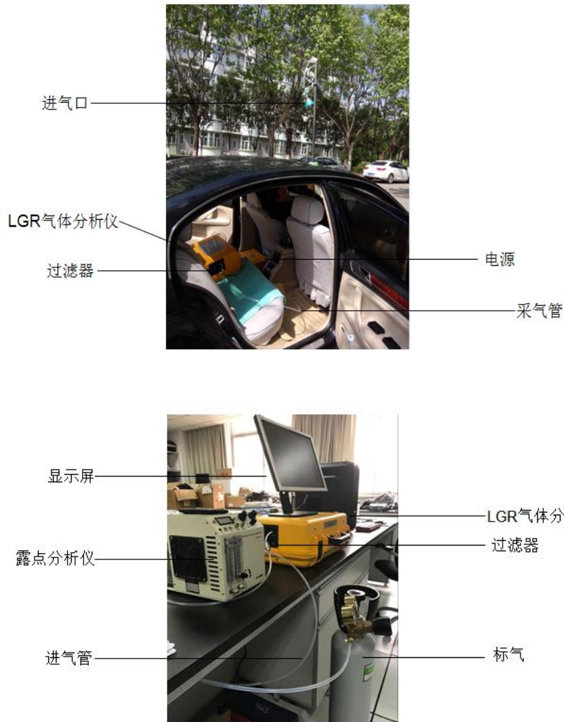
Fig.2 Schematic of instrument installation and calibration
