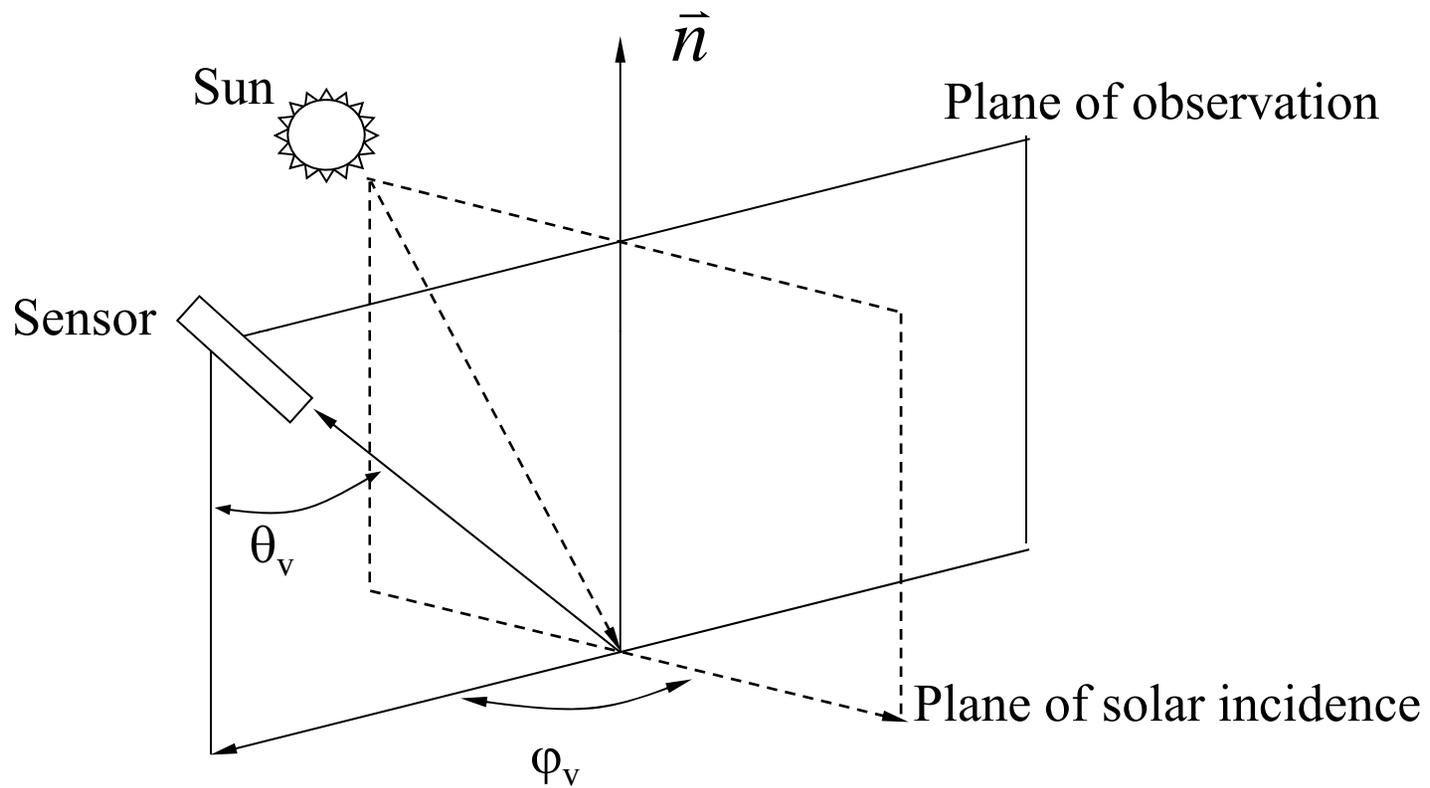
Fig. 2 Viewing geometry of above-water measurement (Tang *et al.*, 2004)
