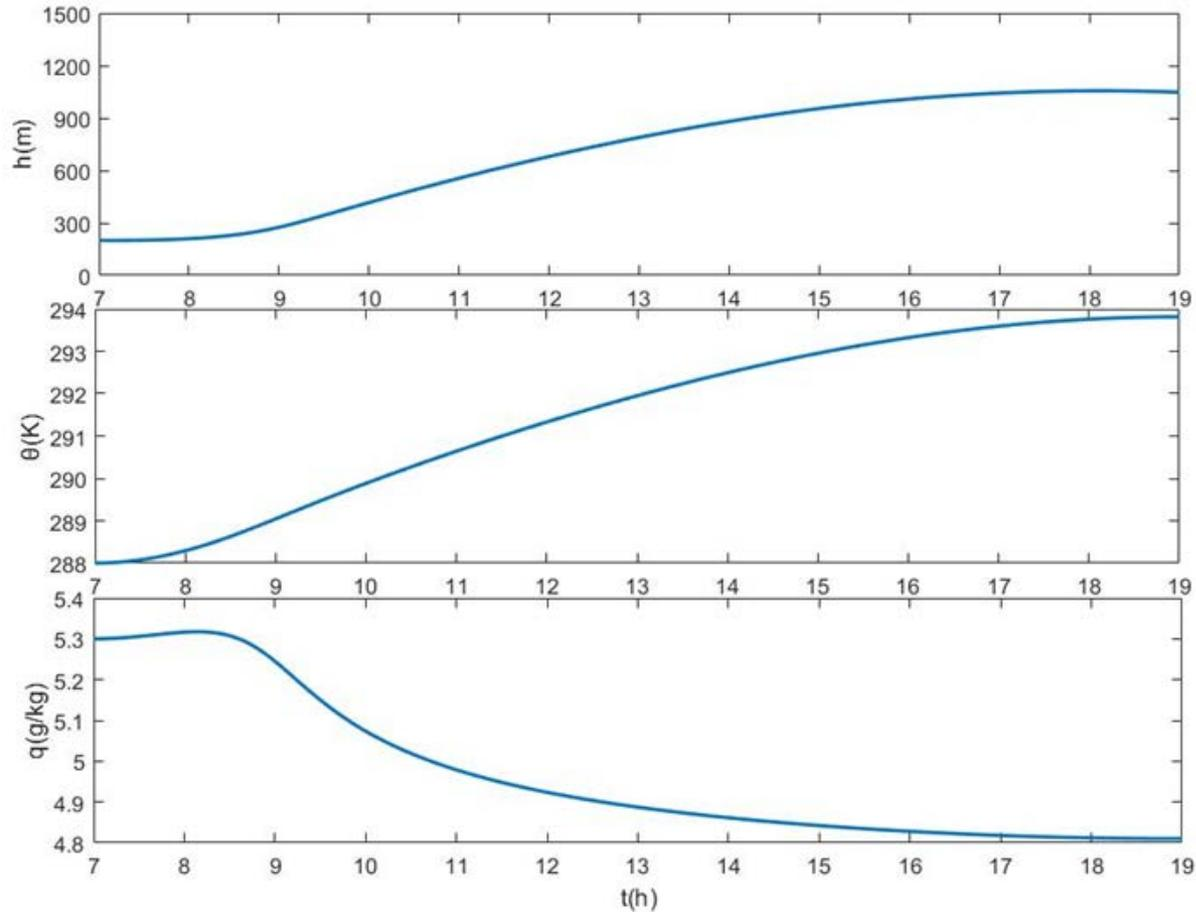
**Fig.7.** The PBL height( $h$ ), potential temperature ( $\theta$ ), and specific humidity ( $q$ ) predicted by CLASS.
