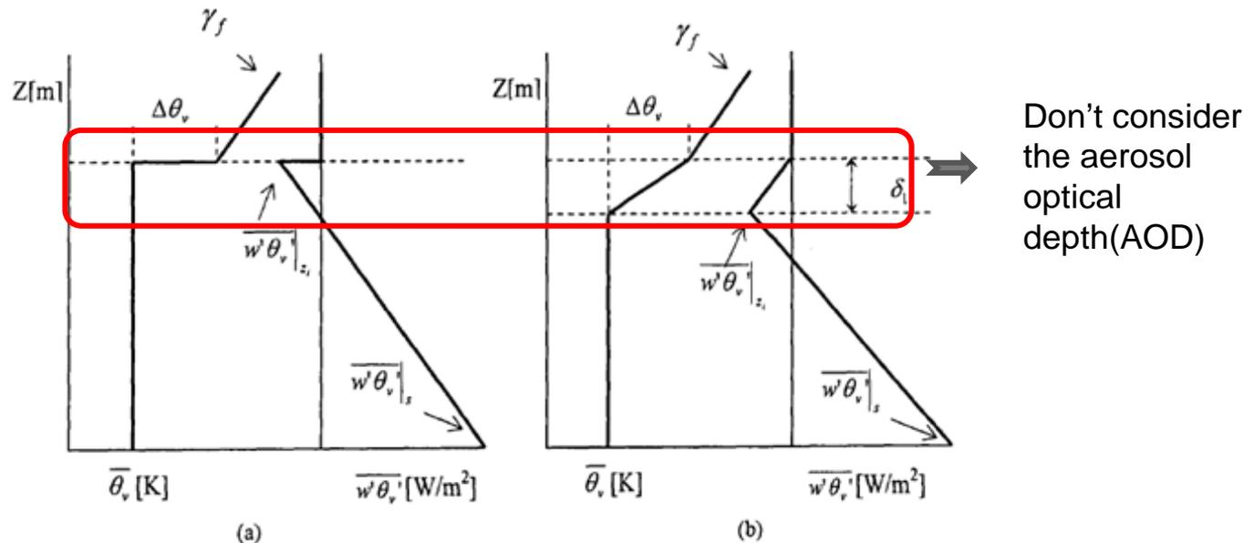
Fig.3. Sketch of the profiles of virtual potential temperature and heat flux in a zero-order and first-order jump model
