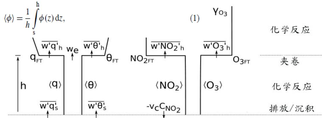
Fig.4. Conceptual representation of the vertical profiles of specific humidity ( $q$ ), potential temperature( $\theta$ )and, as an example, nitrogen dioxide( $\text{NO}_2$ )and ozone( $\text{O}_3$ ).
