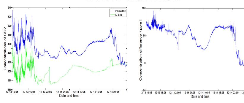
In order to understand the original state of the instrument, before the calibration ,we compared the data of the two instrument. The result is bad.
