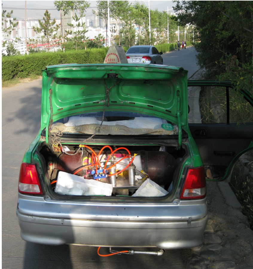
A portable sampling system designed by PM key lab used for on-road test on taxi emission
