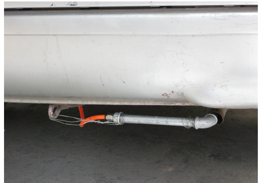
A portable sampling system designed by PM key lab used for on-road test on taxi emission
