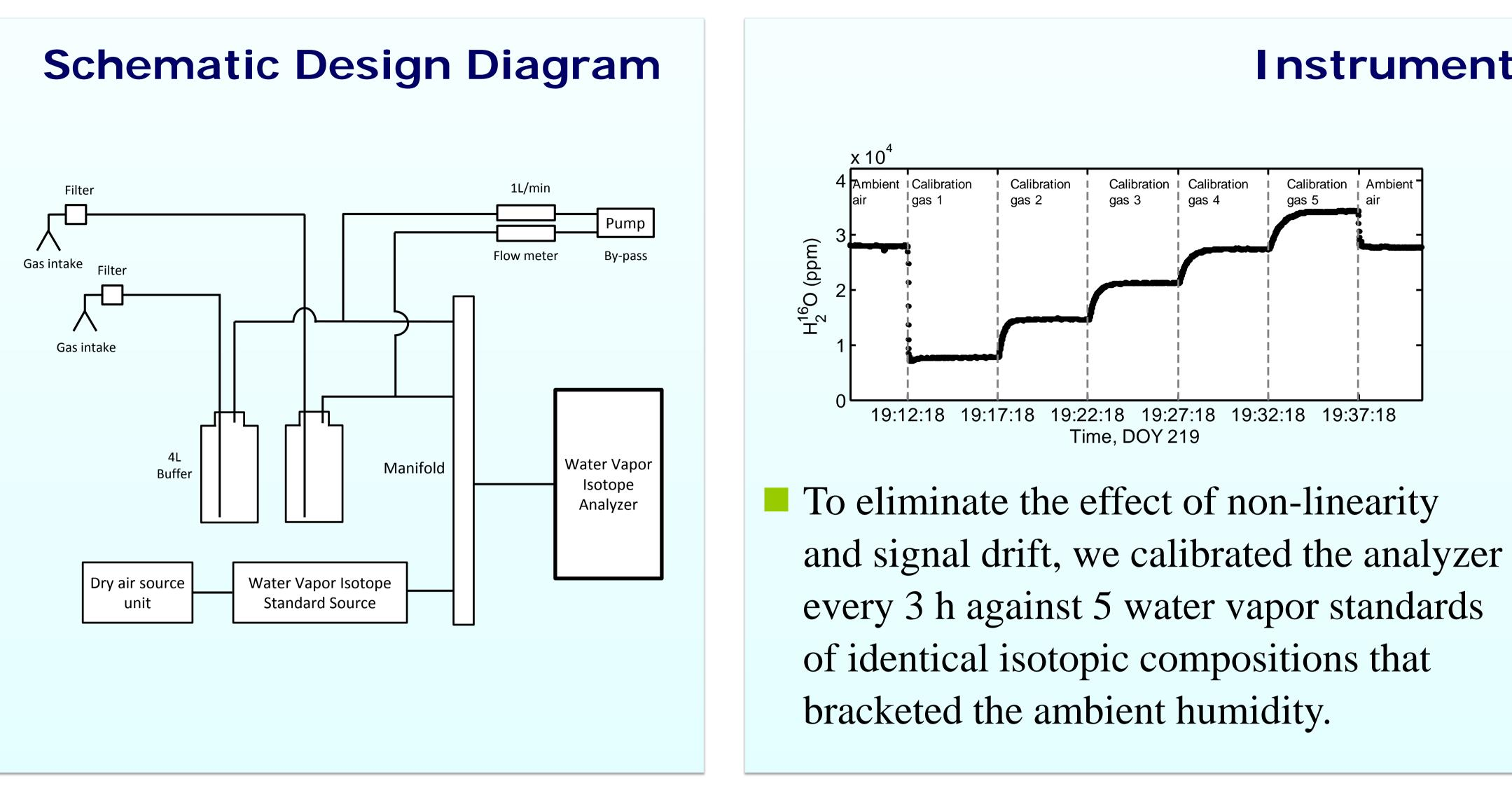
The flux-gradient method was used to obtain the isotopic compositions of lake evaporation.
