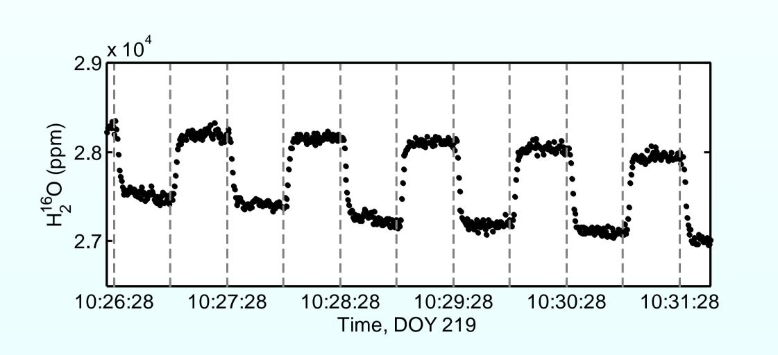
When measuring the ambient air, the manifold switched between the two intakes every 30 s. The measurement approached steady state in less than 10 s after each switching.
