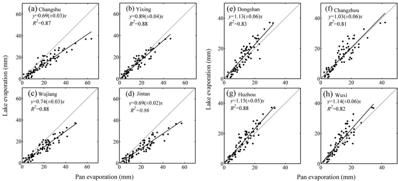
**Fig. 6** Comparison between lake evaporation observed with EC and pan evaporation of four  $\Phi 20$  pans (a–d) and four E601 pans (e–h). Each data point represents a 5-day average in 2012. The pan coefficient of each site is shown as the slope of the regression
