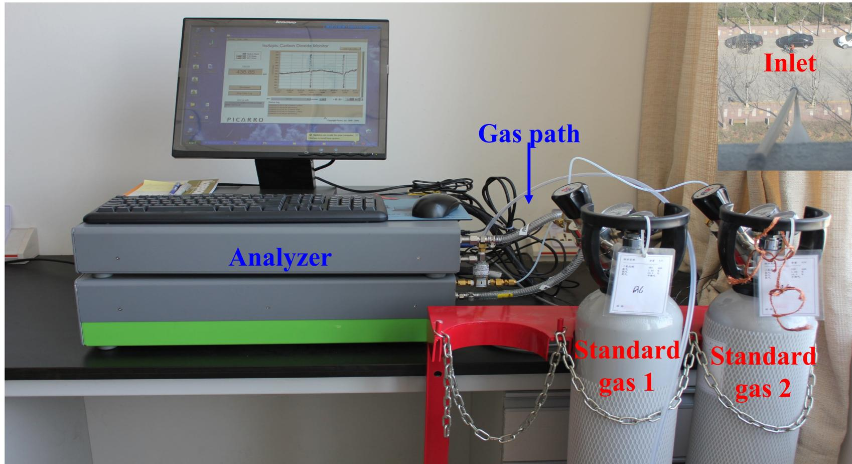
Fig. 1.  $^{13}\text{CO}_2$  analyzer (Picarro G1101-i) and calibration system in Nanjing.
