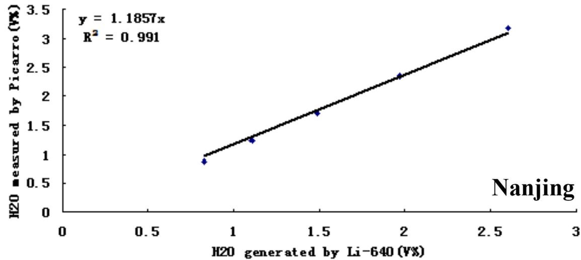
Fig. 3. The relationship between H<sub>2</sub>O measured by Picarro and dew generator Li-640.
