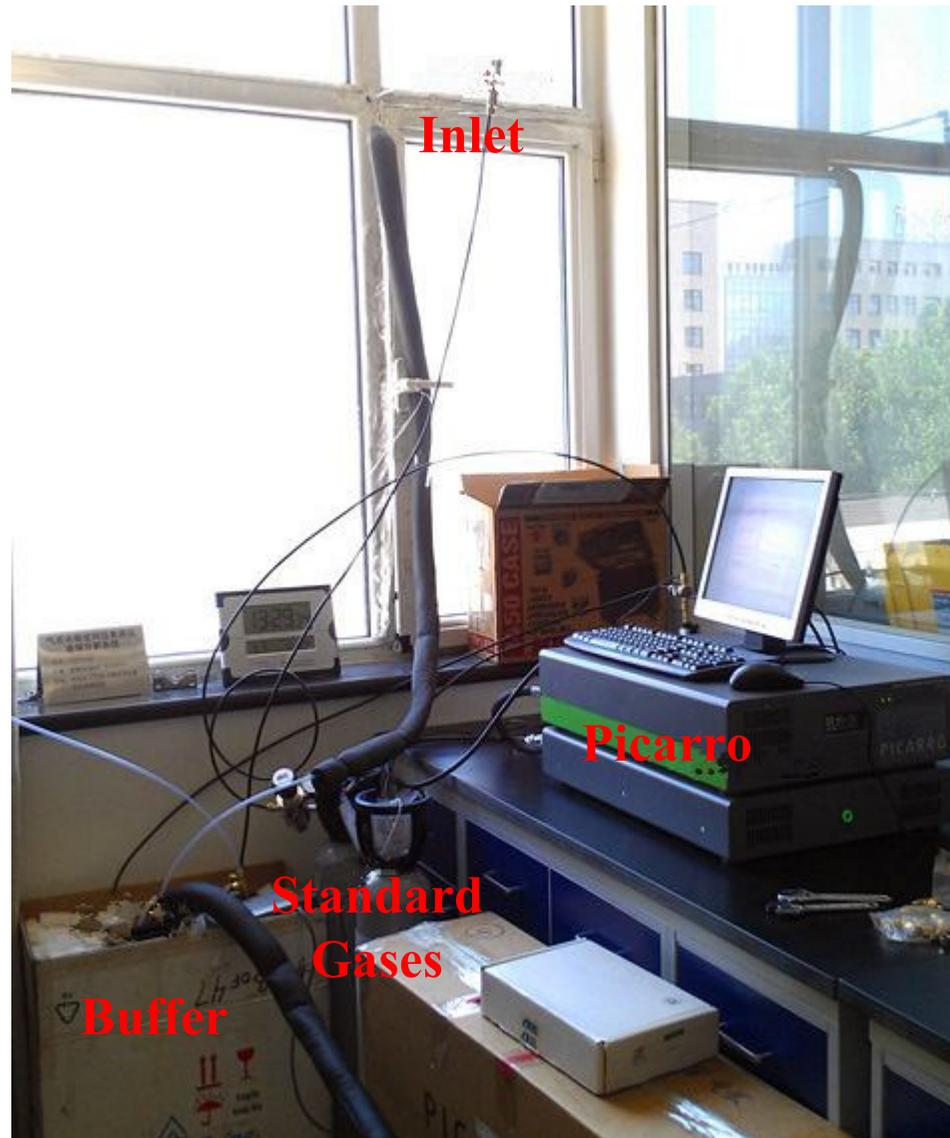
Fig. 2.  $^{13}\text{CO}_2$  analyzer (Picarro G1101-i) and calibration system in Beijing.
