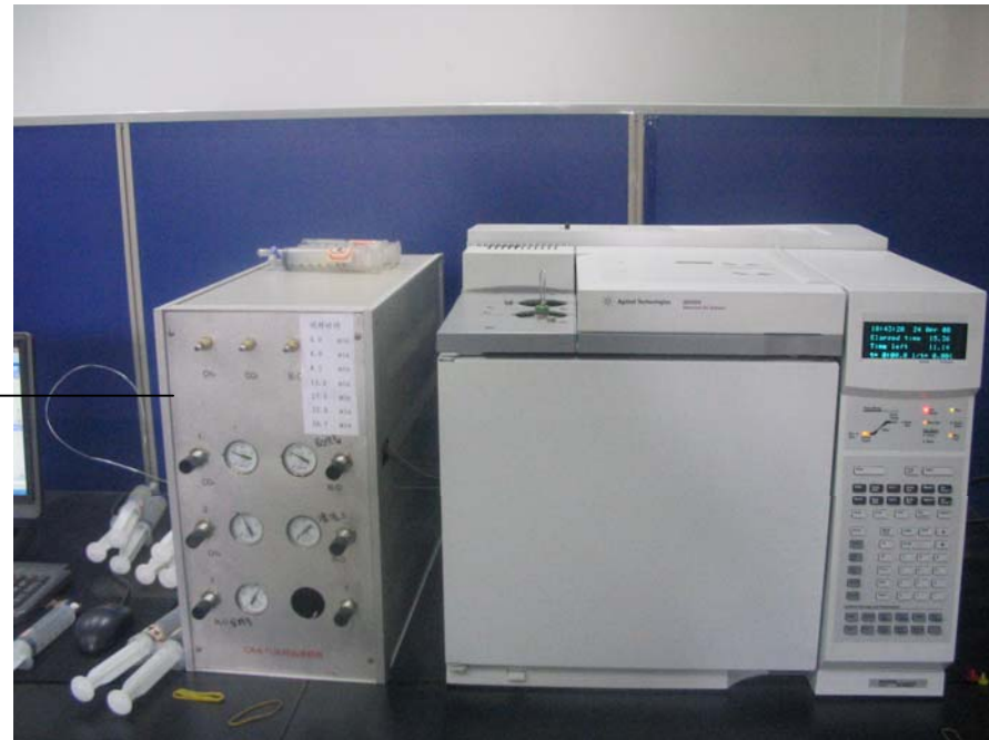
the modified Agilent gas chromatograph
