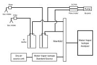
The flux-gradient method was used to obtain the isotopic compositions of lake evaporation. Buffer volumes were used to improve the accuracy of the gradient measurement. Small short tubing was used between the manifold and the analyzer to minimize the transient time between valve switching.
