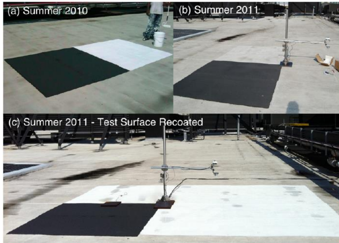
Figure 3. White roof conditions during the summers of 2010 and 2011 showing albedo loss effects over time. The original black membrane was first coated in summer 2009. (a) Surface conditions one year later after a fresh test patch was applied in summer 2010. (b) Surface conditions two years later just before sensor deployment began. (c) Surface conditions at the start of data collection after a second recoating.
