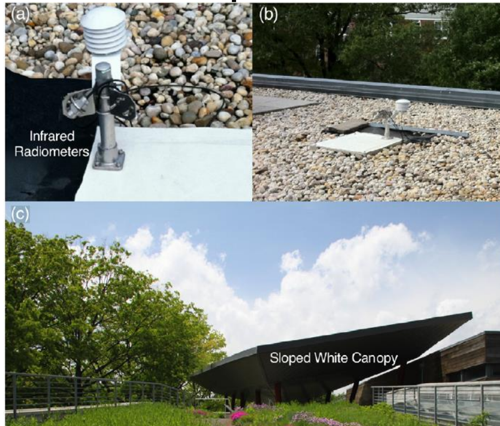
Figure 10. Sensor and test surfaces set up ((a) and (b)) on the Queens Botanical Garden. The building TPO membrane is actually a sloped canopy (c) requiring the use of a small horizontal test membrane.
