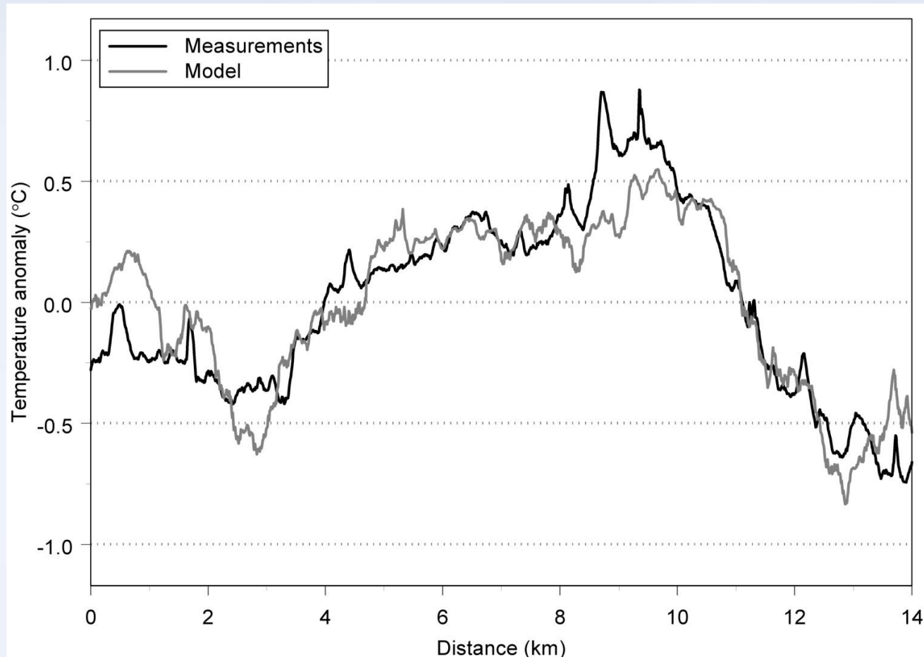
Figure 7: Comparison of the measured and modeled mean nighttime UHI intensity. Anomalies are with respect to profile means.
